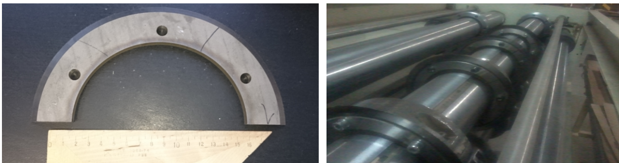
Fig. 4 Paper-cutting knife (a) prepared from the reinforced titanium-based cermet composite and industrial equipment where it tested (b)
