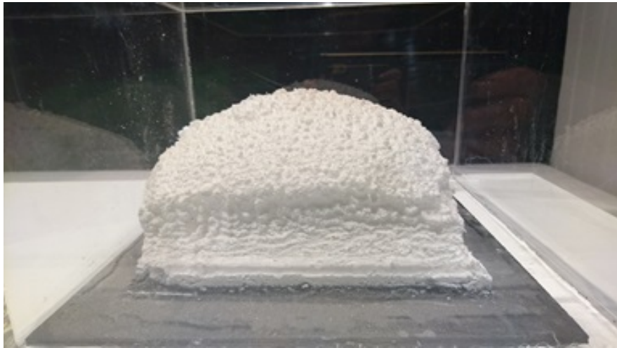
Fig 2. Calcinated foam (the main components are titanium phosphate and silica)
